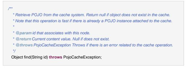
This call will return the current object content located under id. This method call is useful when you don't have the exact POJO reference. For example, when you fail over to the replicated node, you want to get the object reference from the replicated cache instance. In this case, PojoCache will create a new Java object if it does not exist and then add the cache interceptor such that every future access will be in sync with the underlying cache store.
